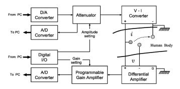
Fig. 2. Experimental setup for the skin-impedance measurement with threeelectrode configuration. The current waveform constructed from PC is applied and the developed voltage is measured. Both the current and voltage are sampled with 20 kHz sampling rate.
