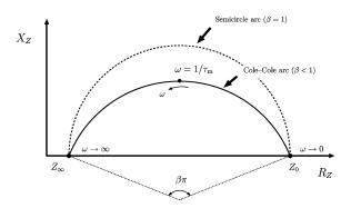
Fig. 1. General impedance locus and corresponding impedance parameters. Note that  $Z_0$ ,  $\tau_m$ ,  $\beta$ , and  $Z_\infty$  indicate the dc resistance, the central relaxation time, the deviation from Debye type ( $\beta = 1$ ) semicircle, and the impedance at infinite frequency, respectively.
